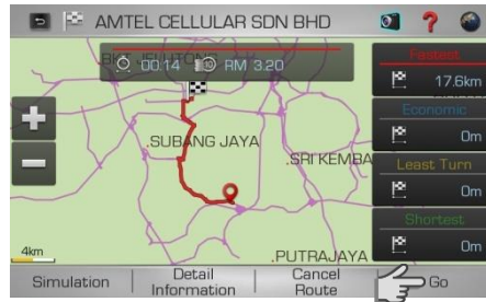
3. Screen will display route information such as the estimated journey time, toll charges and distance for each routing method selected.
